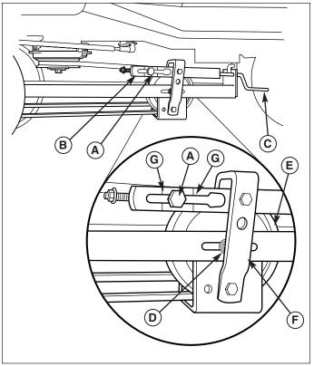
Figure 26. Adjusting Belt Tension
